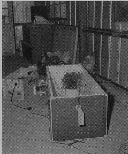
Figure 1. Over-all view of opened chamber, showing exhaust tube, intake, baffle, and watering tubes, with an example of a clover culture
